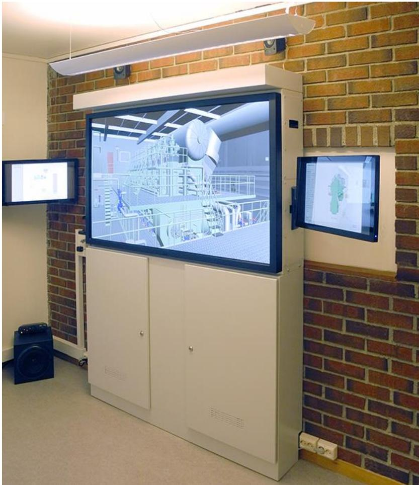
A typical configuration of the Engine Room Simulator with touchscreen solution offers the flexibility in applying different configurations of engine rooms starting from low speed main engine (with conventionally and electronically controlled solutions), through medium to high main engines.
