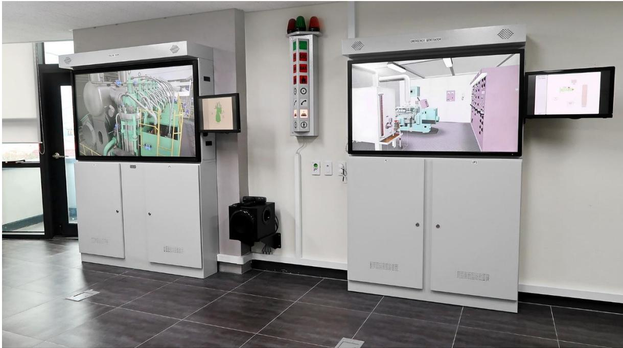
The solutions developed by UNITEST have considerably improved the level of simulator fidelity in comparison to real machinery. In consequence, it was possible to eliminate the disadvantages of the engine room simulator with typical 2D presentation consisting of a schematic and simplified presentation of machinery systems.
